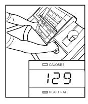
tacts—avoid moving your hands. When your pulse is detected, the Heart Rate indicator will flash, three dashes (---) will appear in the main display, and then your heart rate will be shown. For the most accurate heart rate reading, continue to hold the contacts for about 15 seconds.
